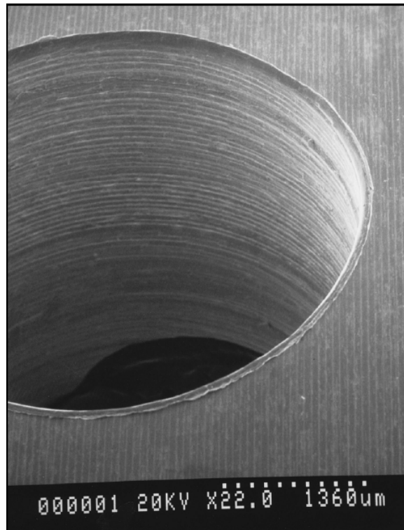
Figure 3.10: SEM Photograph of Seal Drive Pin Hole Prior to Pinning
