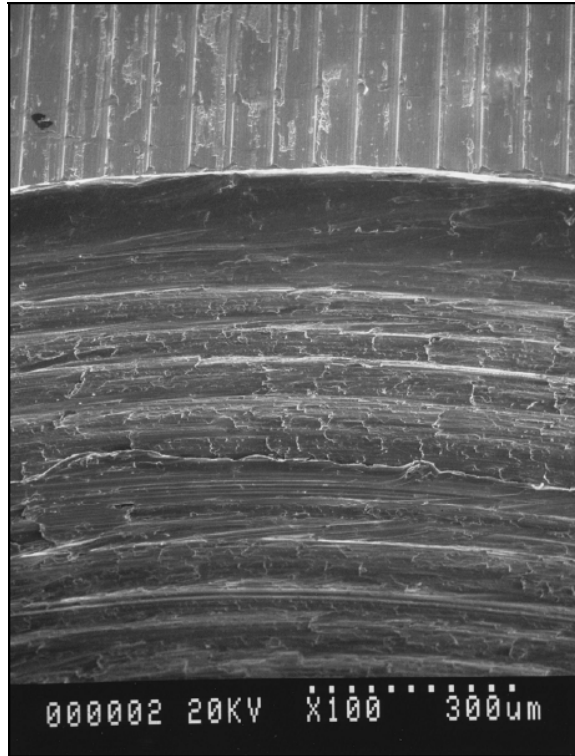
Figure 3.11: SEM Photograph - Closer Examination of Seal Drive Pin Hole
