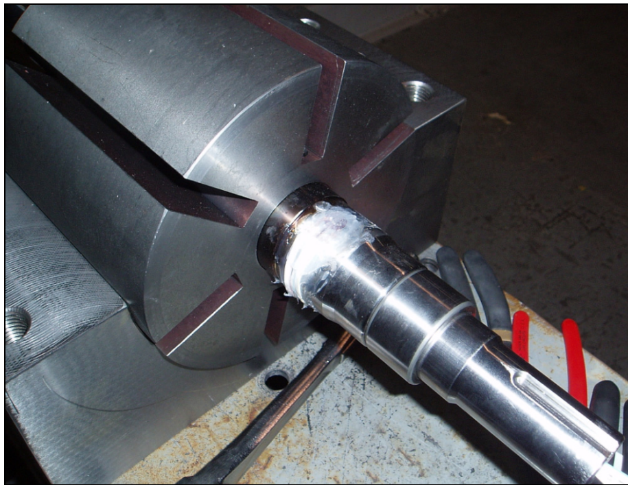
Figure 3.25: Photograph of Strain Gauge with Protective Coating
