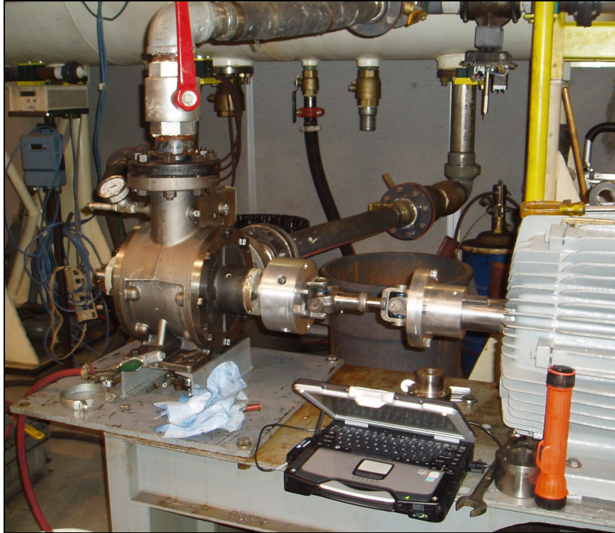
Figure 3.37: Photograph of U-Joint Setup
