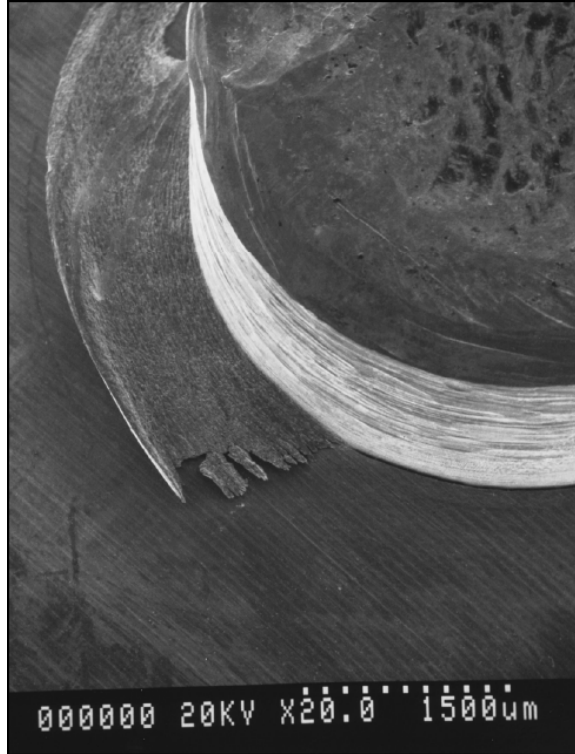
Figure 3.14: SEM Photograph of Seal Drive Pin Hole After the Pinning Operation Showing a Shaving From the Pin
