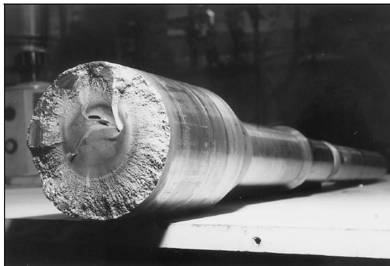
Figure 2.3: Photograph of Nuclear Power Plant Pump Shaft Fracture
