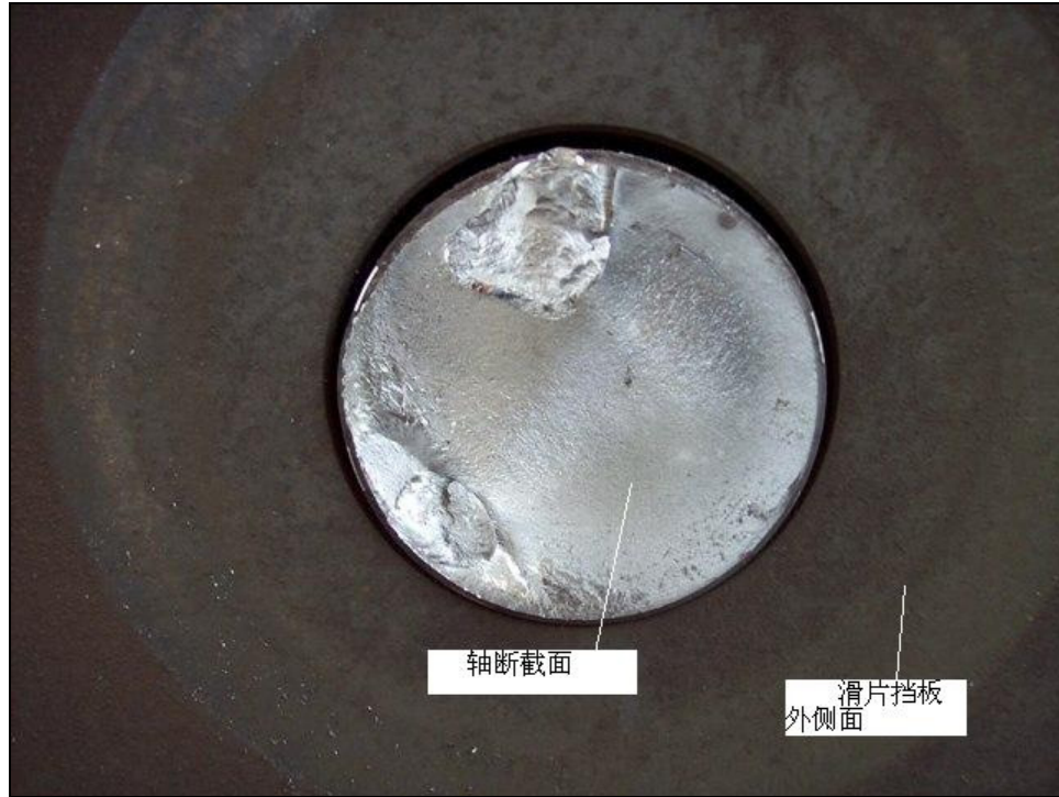
Figure 1.3: Photograph of Typical Pump Fracture Surface Rotor Side
