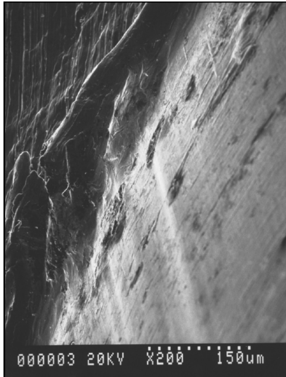
Figure 3.13: Closer Examination of Seal Drive Pin Hole After Pinning
