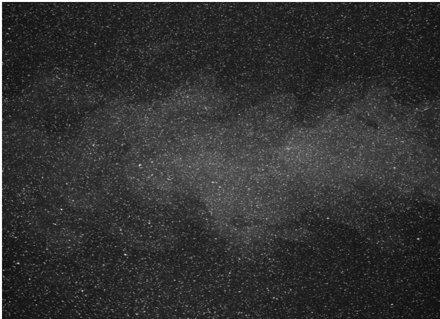
Fig 2.7(b) Second PIV image of jet with particles moving towards right [Westerweel et al. (2005)]
