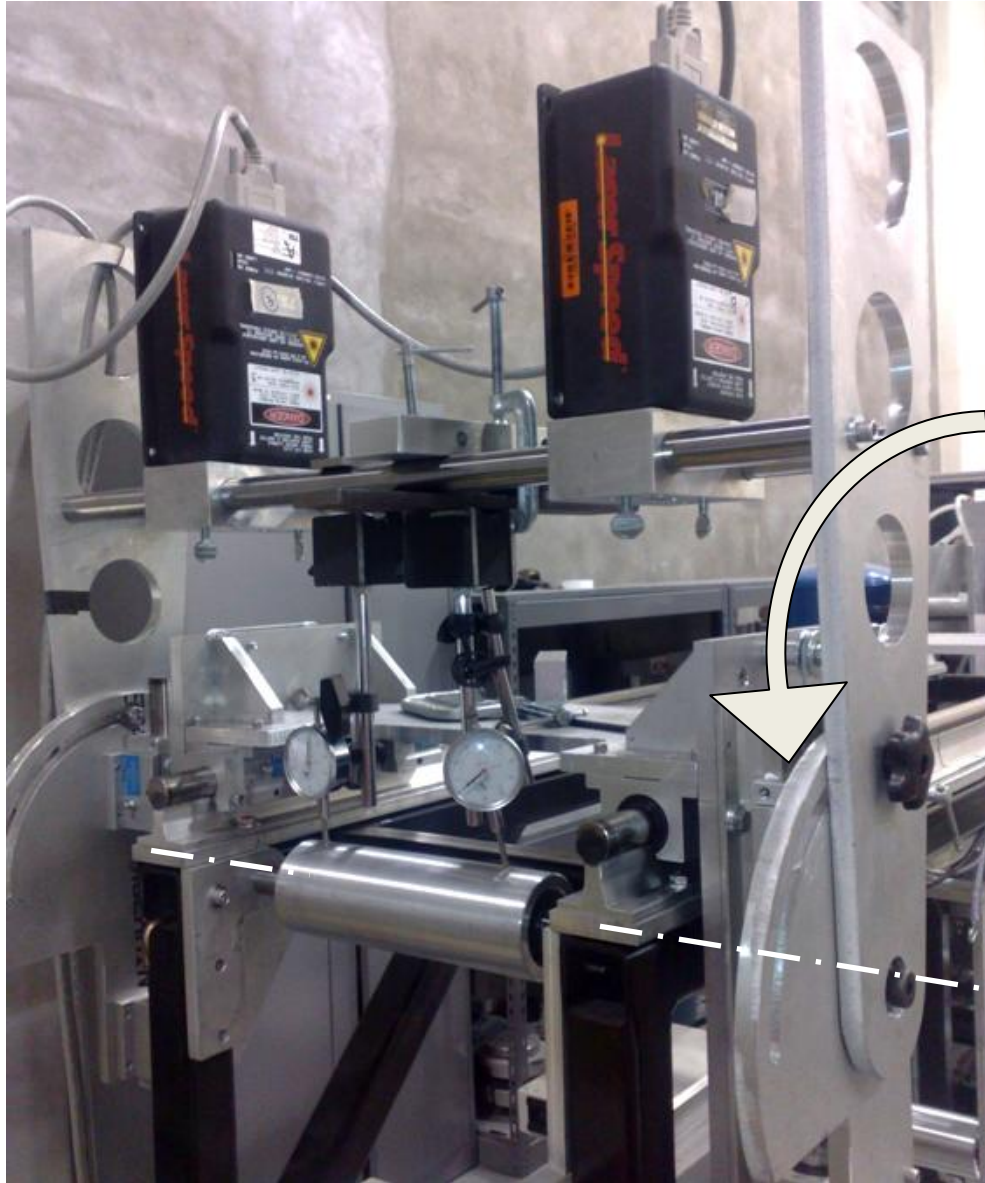
Figure 3.21 Use of Dial indicators for align LDV arm in line to the roller B
