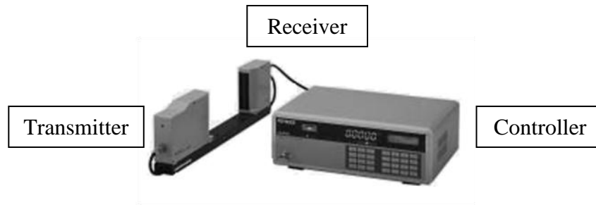
Figure 3.18 A Keyence sensor with its controller
