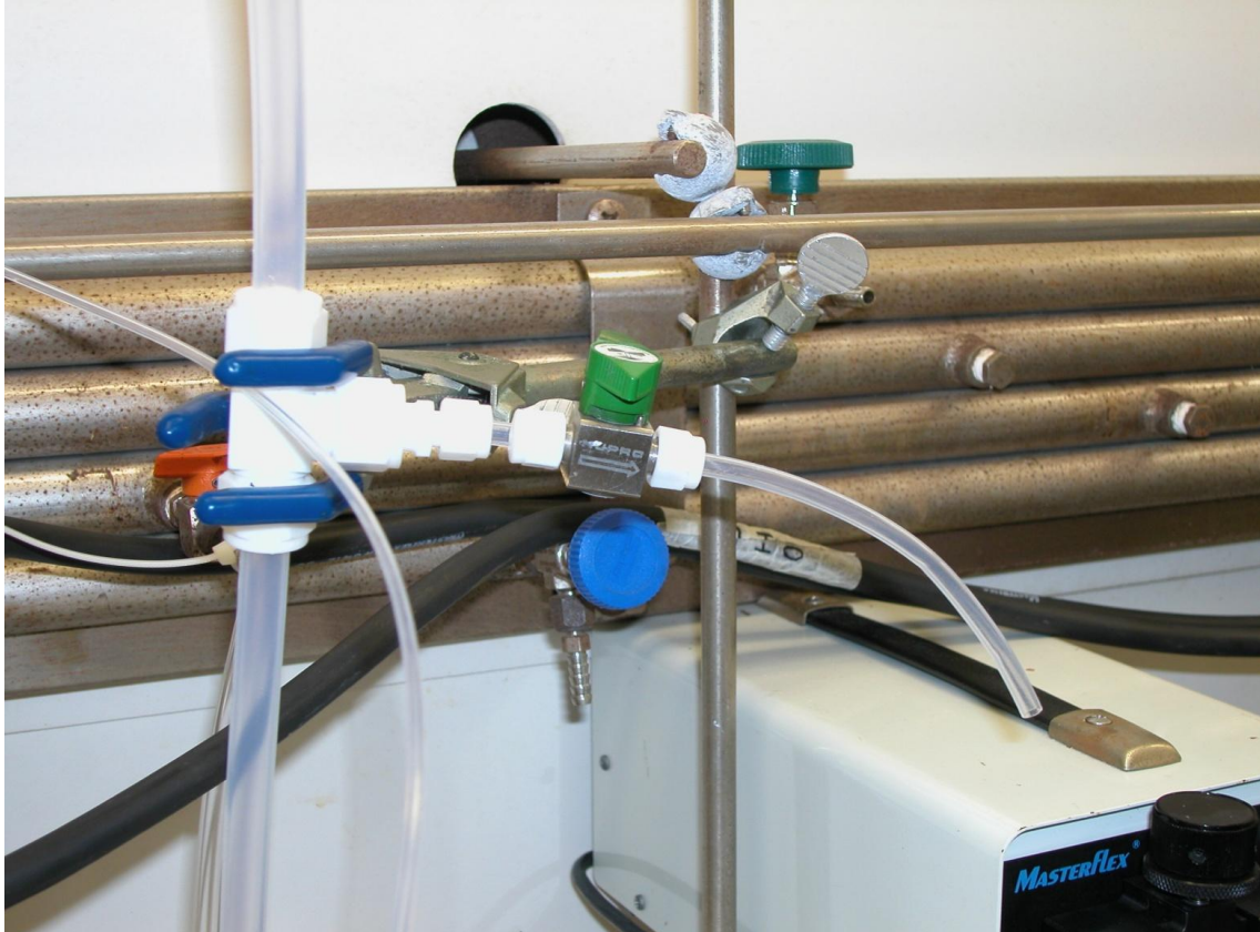
Figure 2.19: Experimental set used to perform off-line sampling (Cho 2010)
