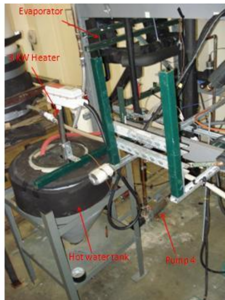
Figure 3-7. Components of evaporator Loop
