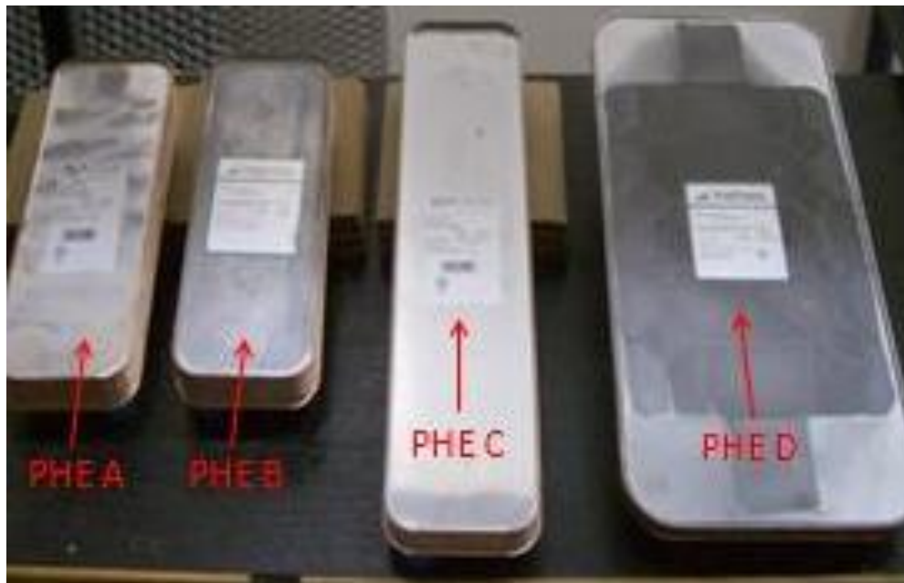
Figure 3-20. Test plate heat exchangers - Condenser-type brazed plate heat exchanger
