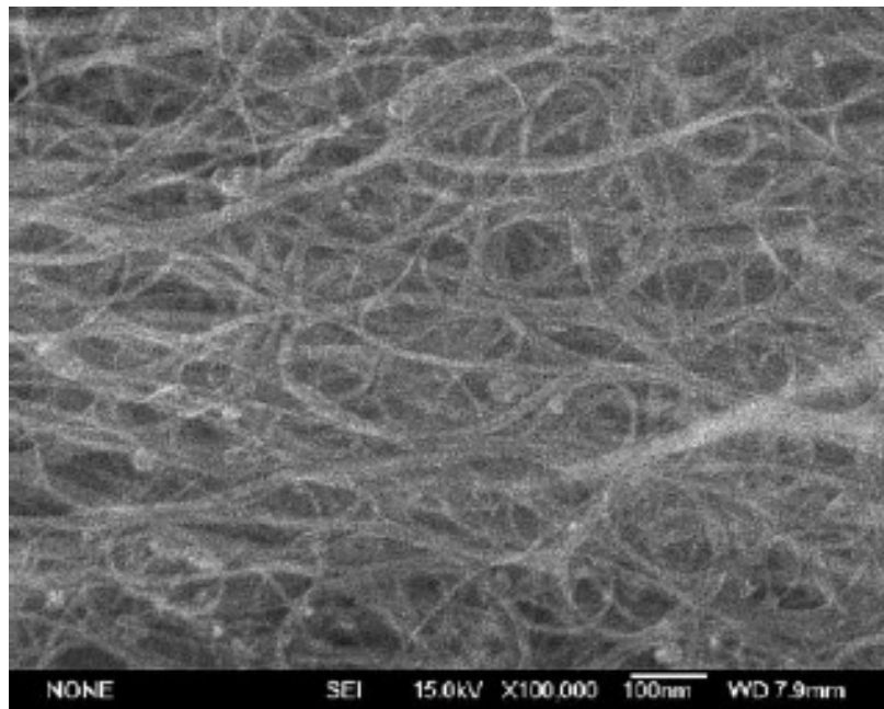
Figure 3.31 SEM micrograph of purified SWNT bundle produced at 600 °C.
