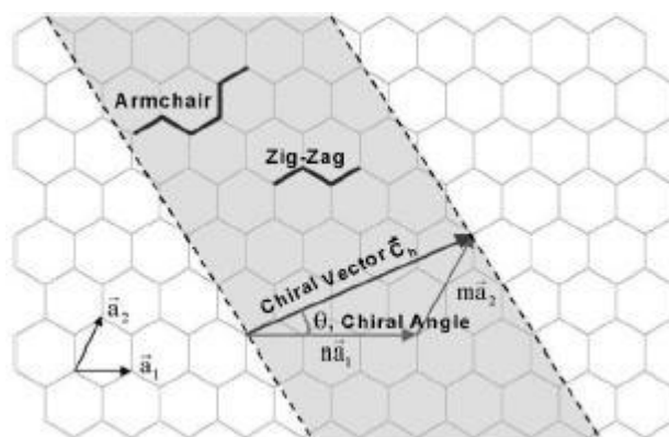
Figure 1.2. Schematic diagram showing the hexagonal sheet of graphite, rolled to form a carbon nanotube [20].
