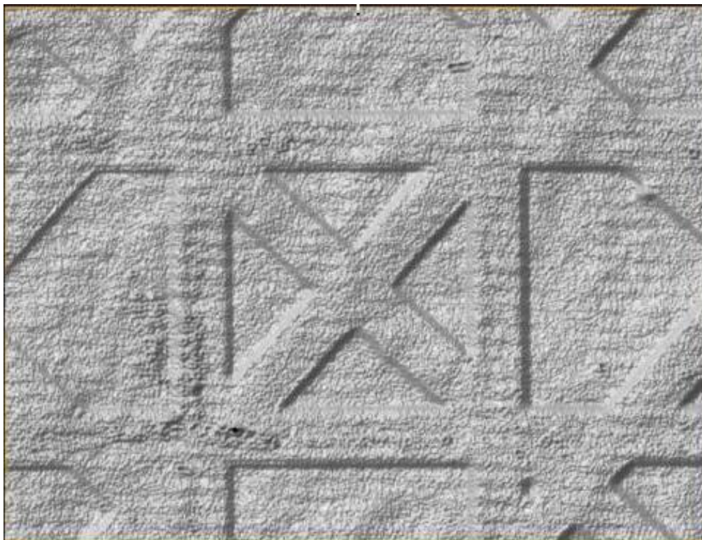
Figure 6.35 MicroXam picture revealing the catalyst pattern
