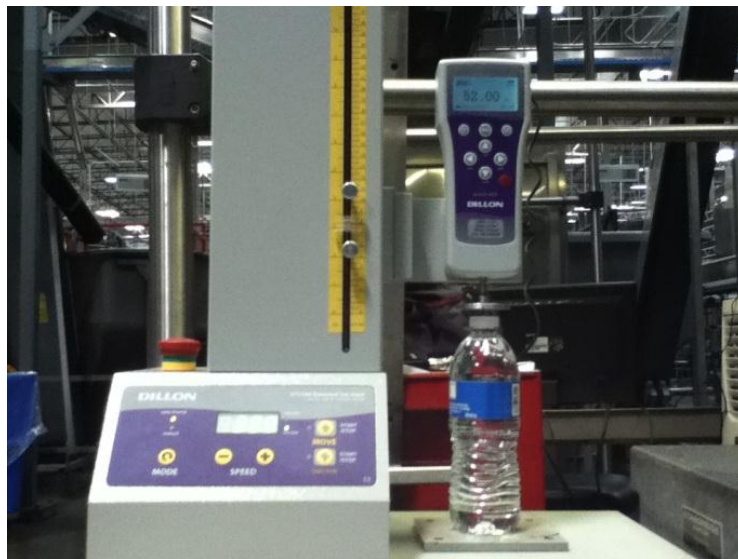
Figure 25: Top load testing setup [138].
