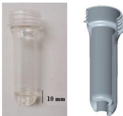
Figure 10: PET tensile preform sample and cross sectional view of CAD model.
