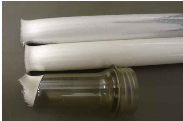
Figure 59: Failed preform samples with crazing after stretching at high extension rate.
