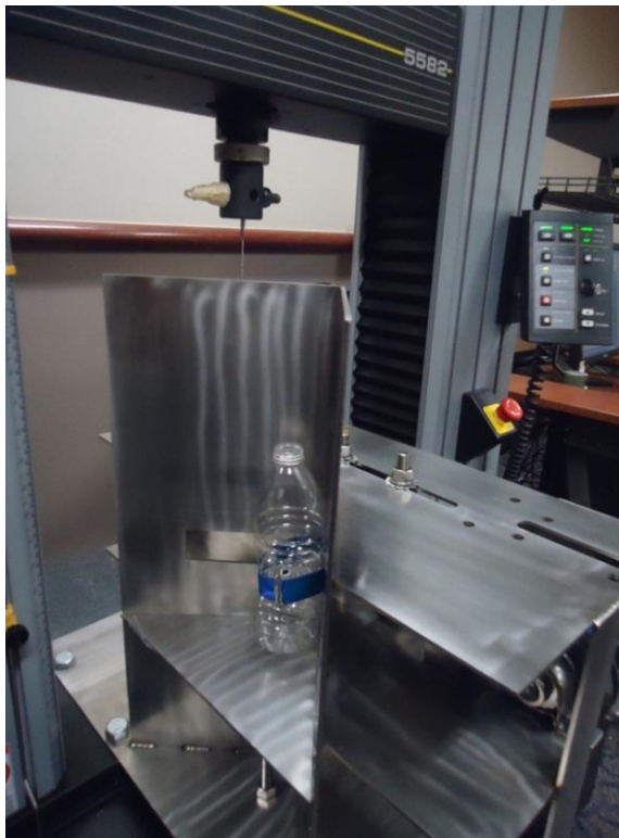
Figure 23: Feel test set up on INSTRON machine.
