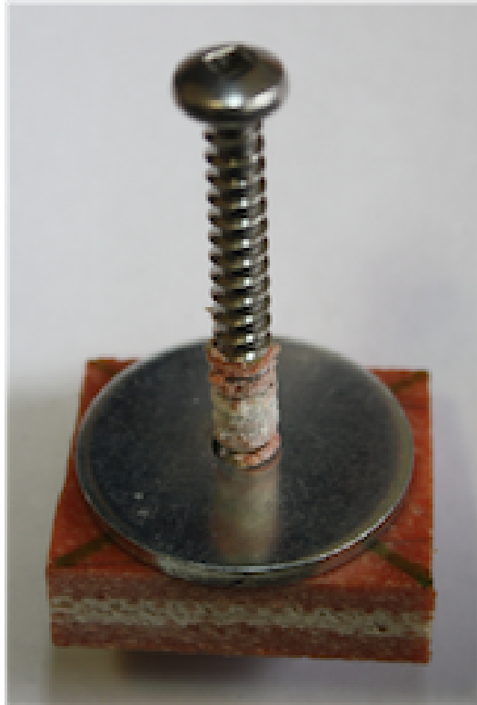
Figure 4.10: Two layer Nylon–SC 79 FBBF laminate with a washer in place
