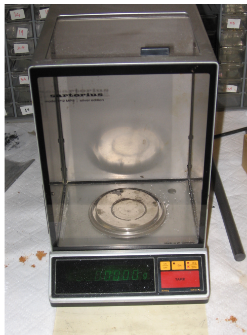
Fig. 5-5: Sartorius manufactured precision digital weighing scale used to measure wafer weight after each polishing cycle.
