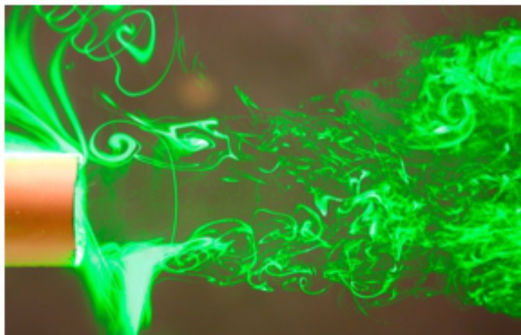
(b) Formation of the turbulent jet as vortex rings evolve
