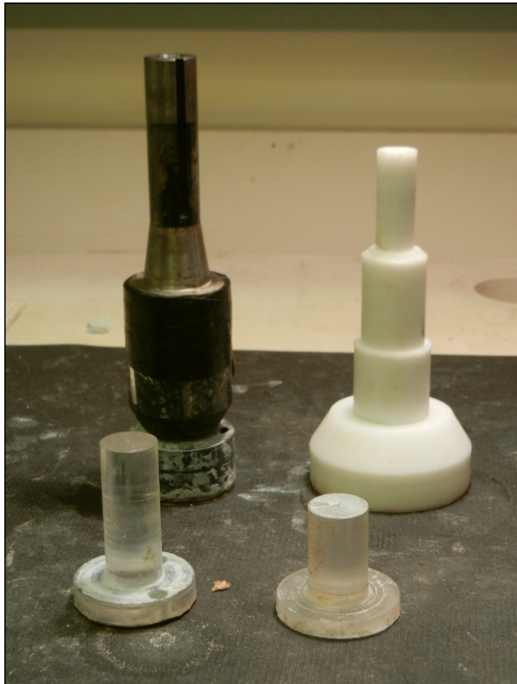
Figure 4.10: Pad holders for different polishing pad sizes used in the multi-stage ECMP
