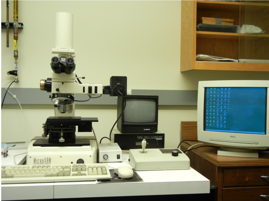
Figure 5.4: MicroXAM, optical laser interference Microscope (from ADE Phase Shift Technologies)
