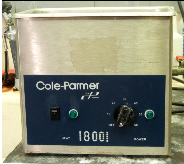
Figure 5.1: Ultrasonic cleaner to clean the copper wafers
