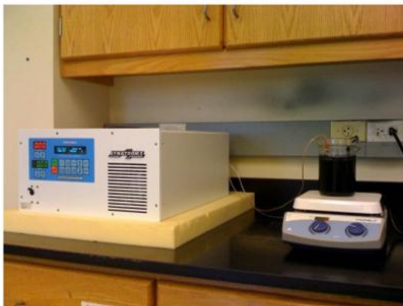
Fig 3.3 Laboratory experimental set-up used for fabrication of Co-W coatings.
