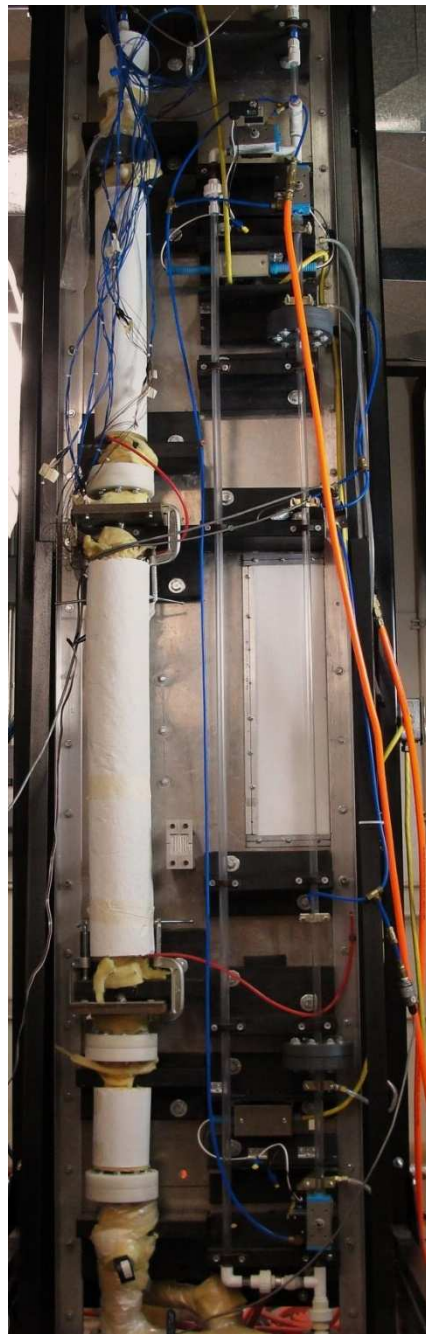
Figure 3.2 Photograph of Experimental Setup and Schematic of Flow Visualization and Void Fraction Sections
