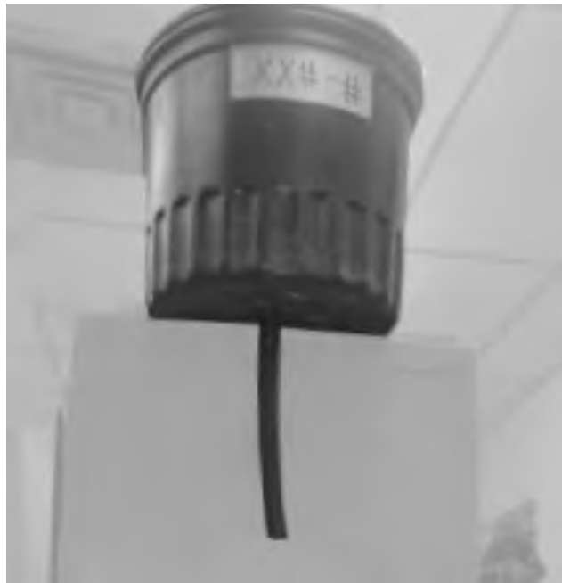
Figure 1: Nursery container (3gal black plastic drain-less) used for laboratory scale Bioretention Cells
