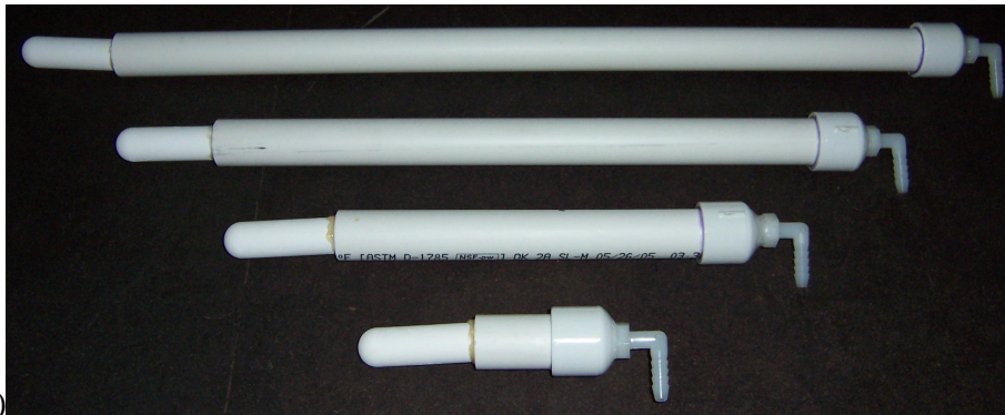
Figure 2. Materials used for lysimeter construction seen in part a.) included A.) a porous ceramic cup, B.) a length of polyethylene tubing, C.) a fitting, and D.)PVC pipe with cap attached. Part B depicts fully constructed lysimeters consisting of a ceramic cup, PVC pipe, cap and fitting. Figure illustrates relative size for 4 depths measured.
