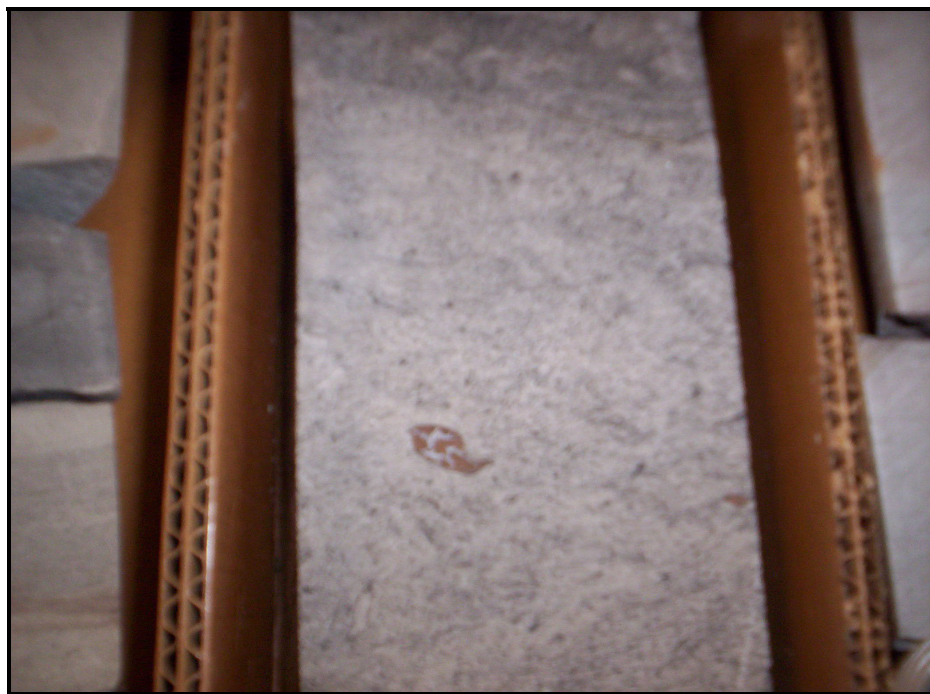
Figure 17: Core photograph of DC-4 deposits of the Bend Group showing some massive and planar bedding.
