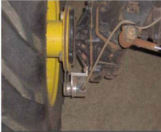
Figure 3.12 Location of Dynapar shaft encoder
