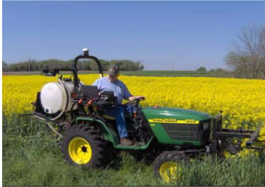
Figure 3.8 John Deere 4100 tractor instrumented with sensors
