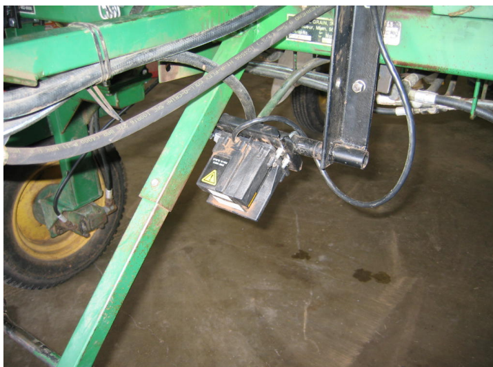
Figure 1. Radar ground speed sensor mounted on the spot sprayer
