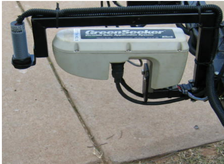
Figure 4. Ultrasonic sensor mounted in front of a GreenSeeker® sensor
