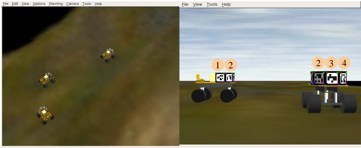
Figure 4.16: Identifications: Robot 1 (right) IDs 2, 3, 4; robot 2 (left) IDs 1, 2.
