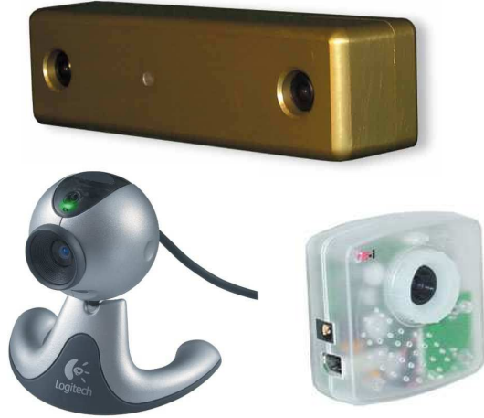
Figure 4.3: Logitech 3000 USB camera (bottom-left), PointGrey's Bumblebee (top), and Unibrain's Fire-I (bottom-right) FireWire IEEE-1394 cameras.
