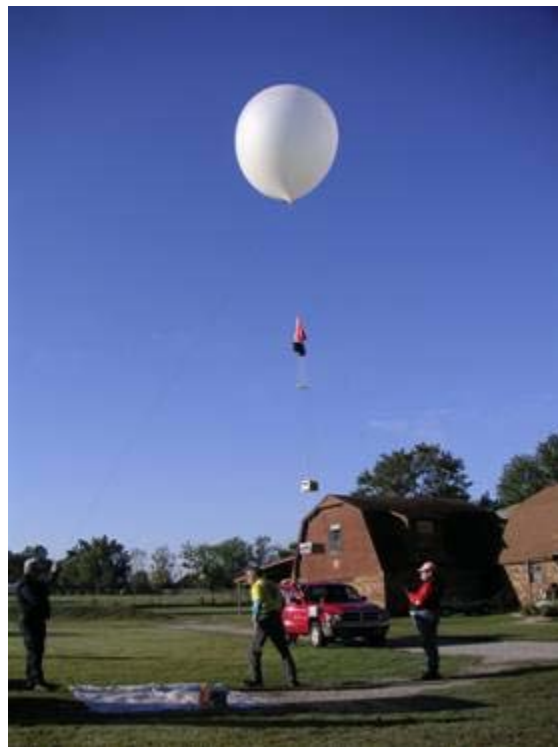
FIGURE A.12: Ozonesonde launch, 08 October 2005; the balloon launch carried the ozone analyzer, two transmitters (for tracking), a camera, and a landing chute.
