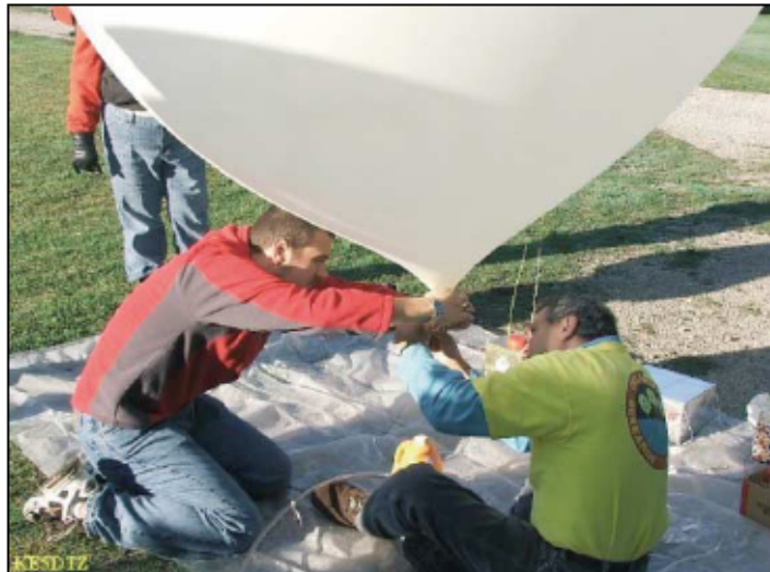
Fig. 1 Preparation of the ozonesonde balloon for launch, 8 October 2005 (© 2005 Scott Mayes)
