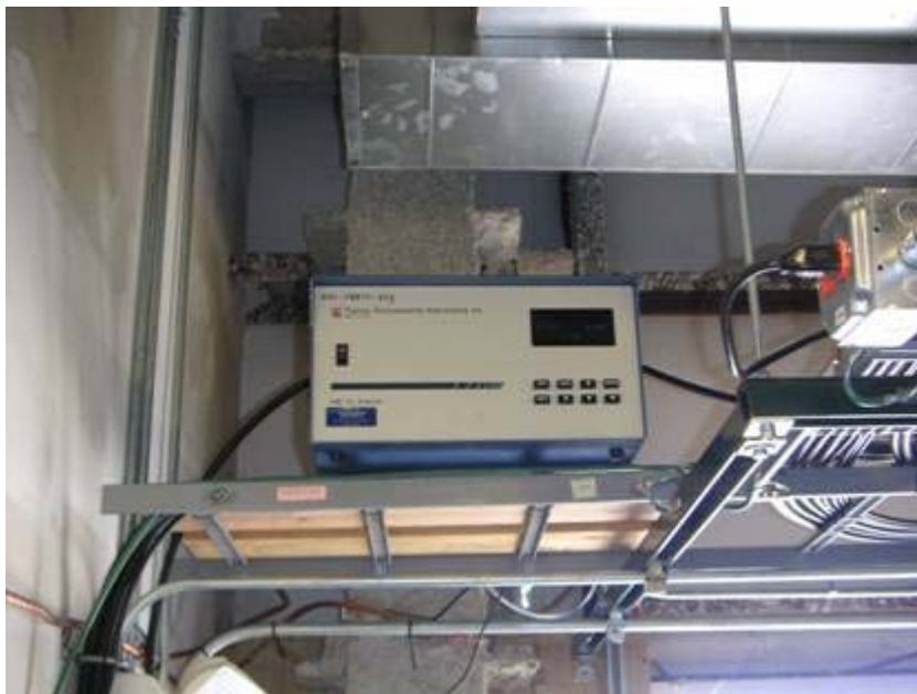
FIGURE A.9: Thermo Electron Corp. Model 49C O 3 Analyzer (front), Bank of Oklahoma Tower; easy access was provided as a result of placement on a communications rack.
