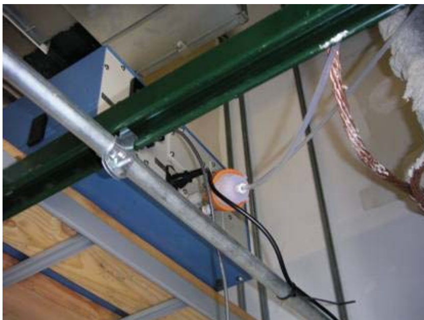
FIGURE A.10: Thermo Electron Corp. Model 49C O 3 Analyzer (back), Bank of Oklahoma Tower; the inlet stream was protected with a particulate matter filter that required replacement every two weeks (orange object).
