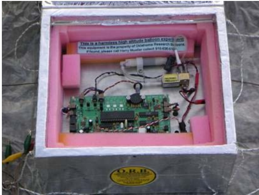
FIGURE A.11: 2B Technologies Model 202 O 3 payload, 08 October 2005 ozonesonde launch; the analyzer and accompanying circuit board were assembled in a padded box for landing protection.
