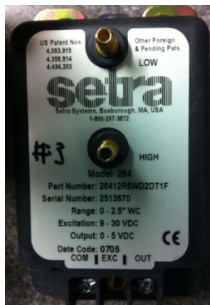
Figure 30: Differential pressure transducer
