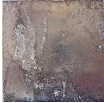
200 ppm Ca(gluconate)borate in 0.5M Cl - soln. for 1 week
