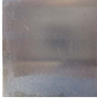
200 ppm \text{Cr}(\text{propionate})_3 in 0.5M \text{Cl}^- soln. for 1 week
