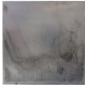
200 ppm \text{CrO}(\text{OH}) in 0.5M \text{Cl}^- soln. for 1 week
