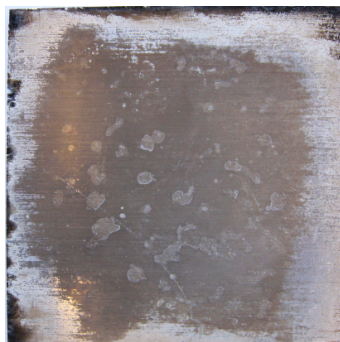
200 ppm \text{K}(\text{benzilate})\text{molybdate} in 0.5 M \text{Cl}^- soln. for 1 week
