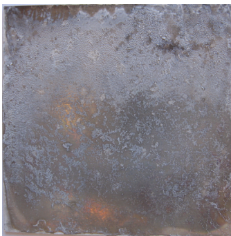
Al 7075 alloy control in 0.5M \text{Cl}^- soln. for 1 week
