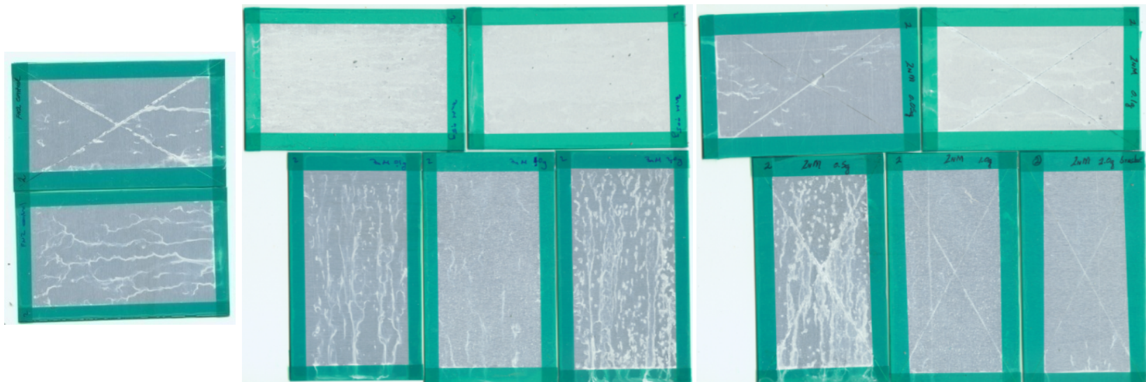
On top from left to right: 0.05 g and 0.5 g zinc mandelate added coupons, respectively. At the bottom from left to right: 0.1 g, 1 g, and 2 g zinc mandelate added coupons, respectively.
