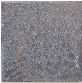
200 ppm \text{Cr}(\text{butyrate})_3 in 0.5M \text{Cl}^- soln. for 1 week
