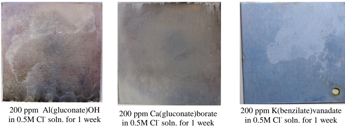
Figure 4-24 Aluminum 6061 coupons immersed in solutions of various inhibitors
