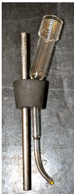
Figure S2: A number six-rubber stopper modified to hold a graphite counter electrode and a luggin probe (bridge tube) for the saturated calomel reference electrode.
