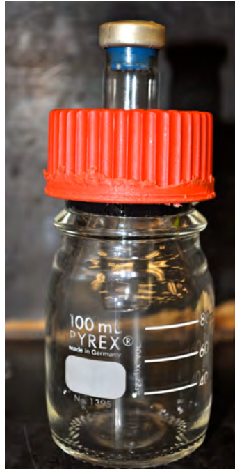
Figure S1: A 100 ml culture bottle used as an electrochemical cell during corrosion experiments with D. alkanexedens strain ALDC and S. aciditrophicus strain SB pure cultures and related co-cultures.
