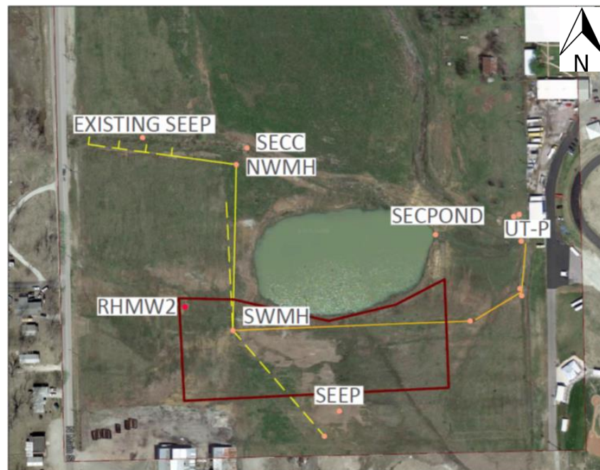
Figure 1.6: SEC post-land reclamation (2015) aerial image with the French drain shown in yellow and future passive treatment system location in red (Google Earth, 2016)
