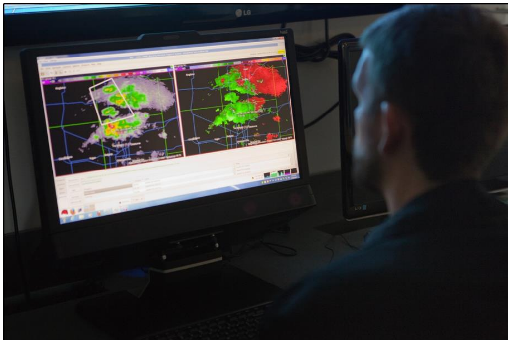
Figure 4.1. Forecaster interrogating 1-min base velocity and reflectivity PAR data using the Warning Decision Support System-Integrated Information. The Tobii TX300 eye-tracker is positioned below the monitor.
