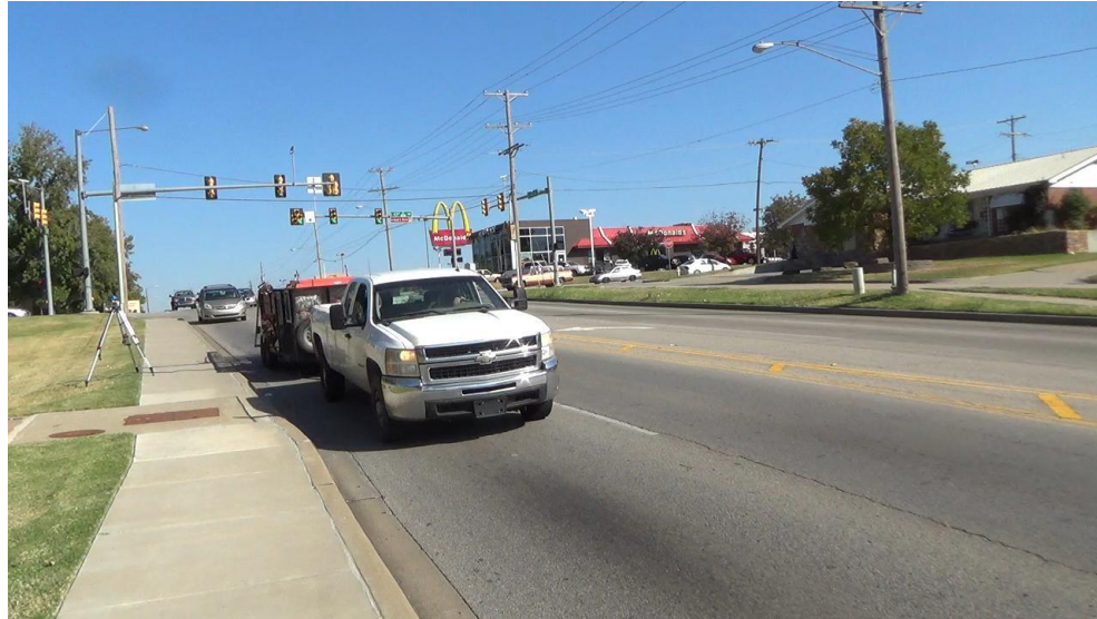
Figure 6-27 Class 3 truck with huge trailer on edge of lane 2, detected in both lanes
