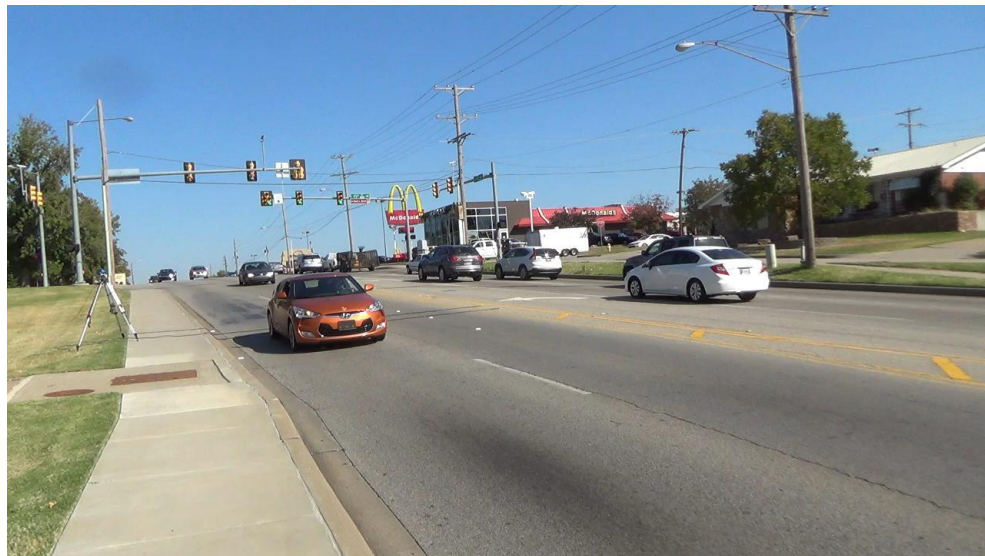
Figure 6-28 Class 2 hybrid car on the edge of lane 2, detected in both lanes
