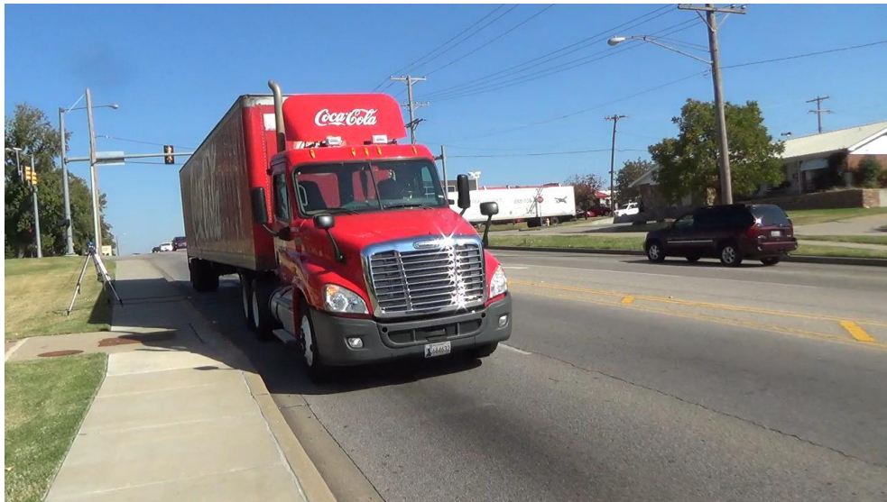
Figure 6-25 Class 9 truck at the edge of lane 2, detected in both lanes
