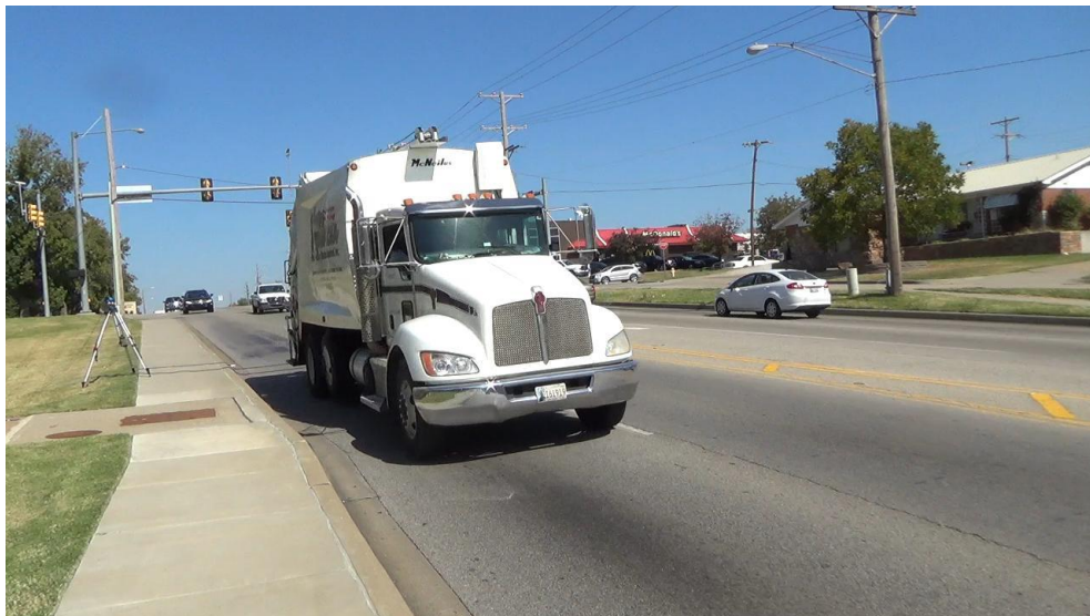
Figure 6-26 Class 6 truck on the edge of lane 2, detected in both lanes
