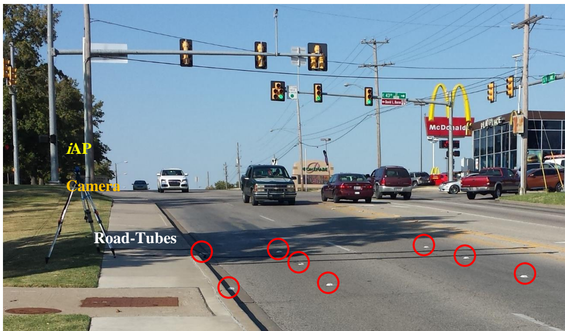
Figure 5-10 Eight iVCCS nodes deployed on an urban road
