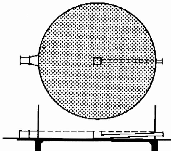
Figure 1. A totally-perforated floor system.
