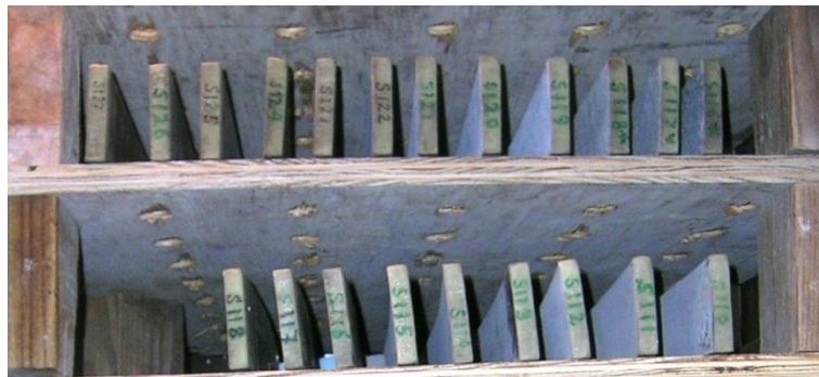
Figure 3 - 2: The specimens covered with curing compounds stored in the chamber room
