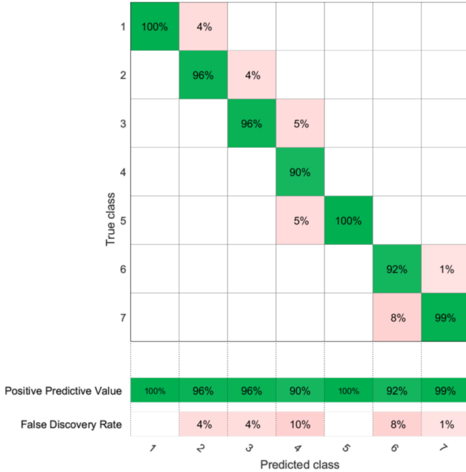
Figure 6.15. Confusion matrix for the binary decision tree classifier. Classes one through seven represent transmitter power level.
