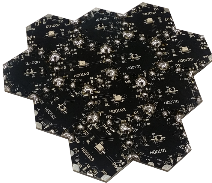
Figure 4.11. 12-module flat array with 850nm detectors (solid white) and 940nm detectors (white with black dot).
