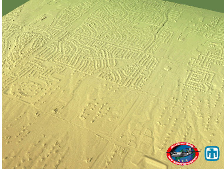
3-D Rendering of Northeast Albuquerque, NM Created from RTV DEM (DTED Level IV)
