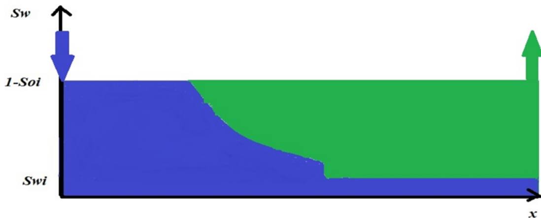
Figure 4- 18: Non-ideal water flooding- The tongues of the displacing fluid (water) are bypassing the displaced fluid (oil).
