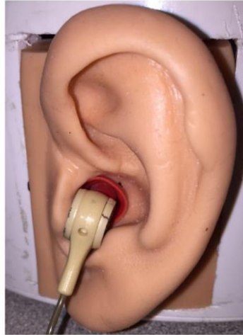
Figure 28: Combat Arms EP inserted into scale ear model. [Shows the third of the triple-domes blocking, but not entering the ear canal.]
