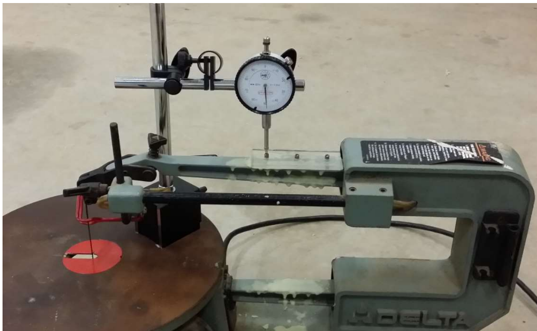
Figure 3-7: Vertical Displacement of Saw Arm Measurement
