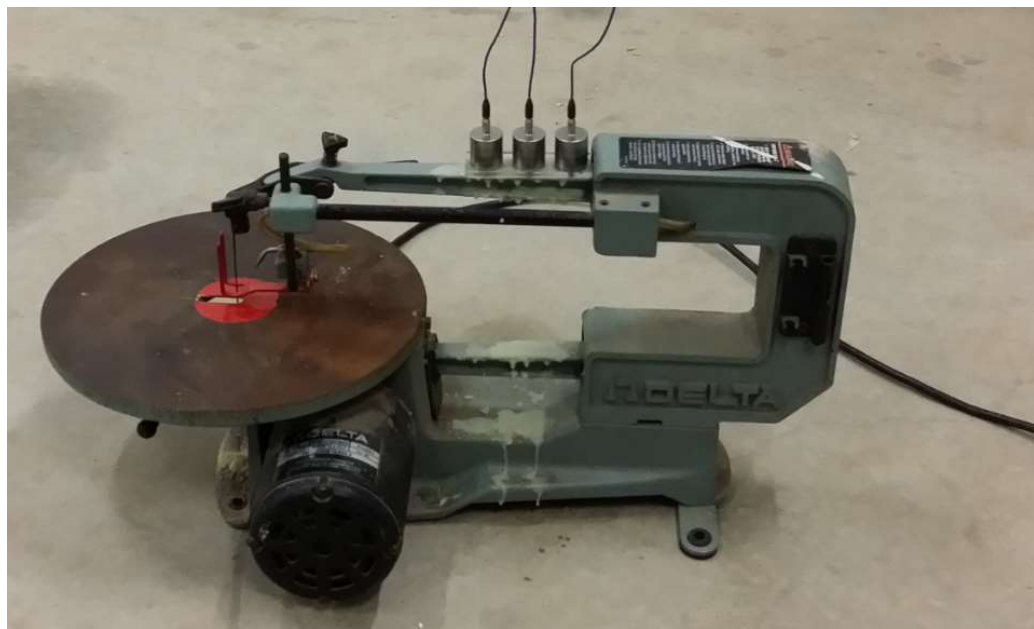
Figure 3-6: Scroll Saw with Sensors Attached
