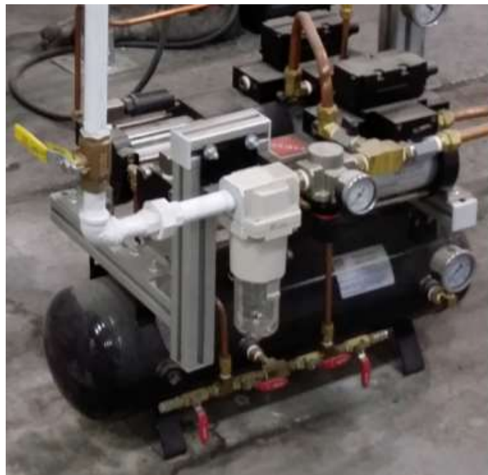
Figure 4-24: Picture of Compressed Air Booster
