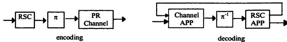
Figure 2.7. Serial concatenation of a PR channel and a convolutional code.
