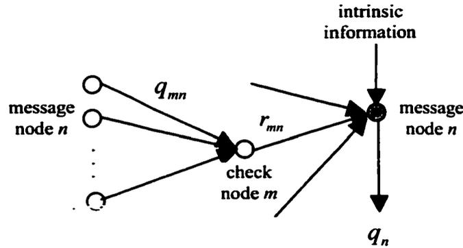
Figure 4.4. Message flow in the BP algorithm.
