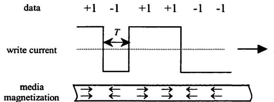
Figure 1.1. Illustration of data, write current and magnetization pattern.
