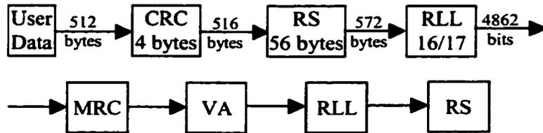
Figure 5.7. An RS coded system.
