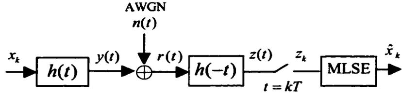
Figure 1.6. Optimal detector for ISI channel with AWGN.
