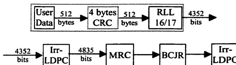
Figure 4.18. System diagram using an irregular LDPC code.
