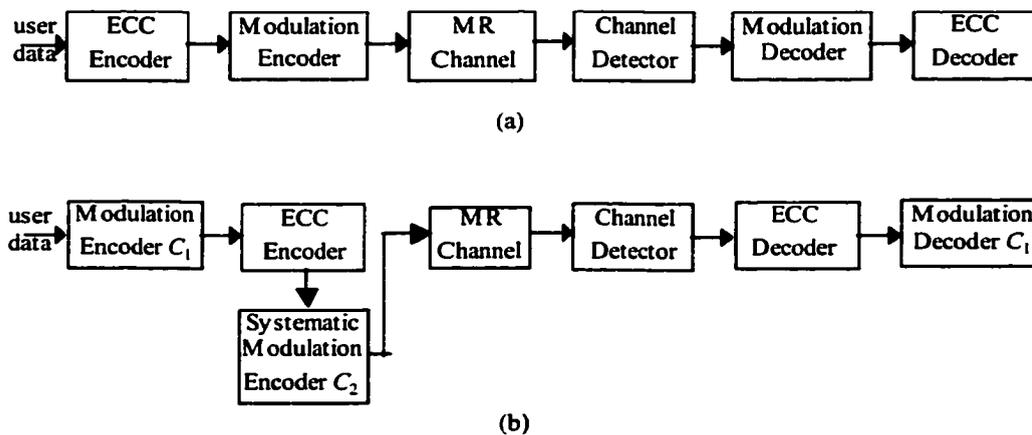
Figure 2.4. Concatenation of ECC and modulation code. (a) standard concatenation; (b) modified concatenation with a second systematic code.
