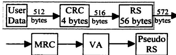
Figure 5.8. Model for an RS coded system.
