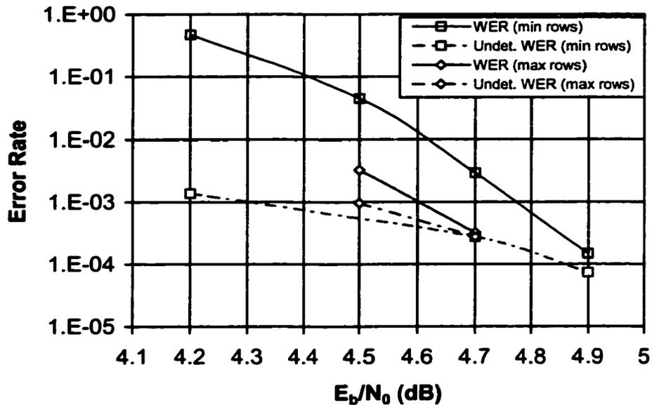
Figure 4.15. Performance of C-EG(3,2<sup>3</sup>) on AWGN, with different redundancy parity check matrices. Maximum 50 iterations.
