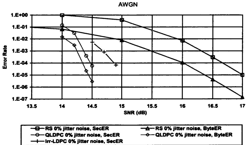
Figure 5.10. Performance on channels with purely AWGN.
