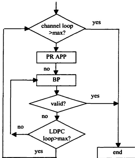
Figure 4.6. The flow chart for iterative decoding.
