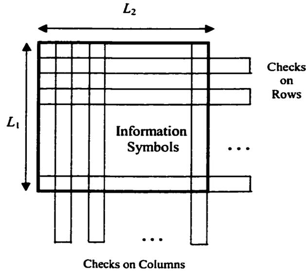
Figure 3.2. Construction of parallel concatenated block codes.
