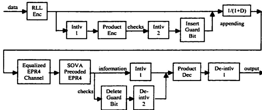
Figure 3.5. Diagram of an equalized EPR4 MR system with a product code.
