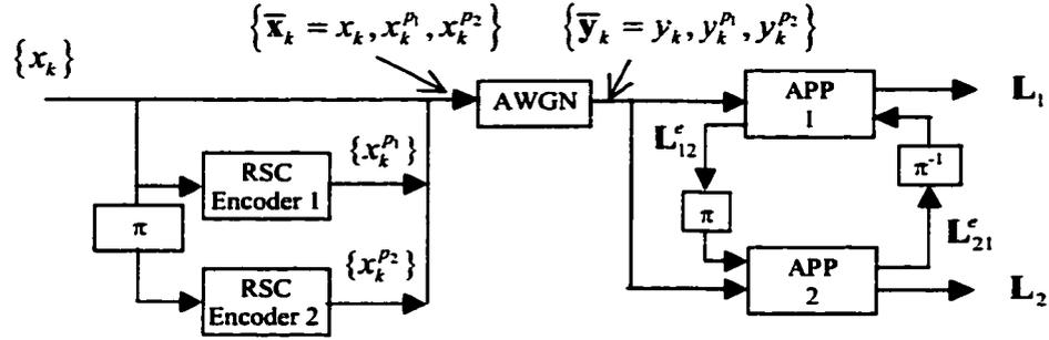
Figure 2.5. Turbo coding and decoding.
