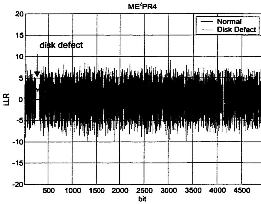
Figure 5.12. Equalized ME<sup>2</sup>PR4 channel BCJR output with 80-bit full erasures.
