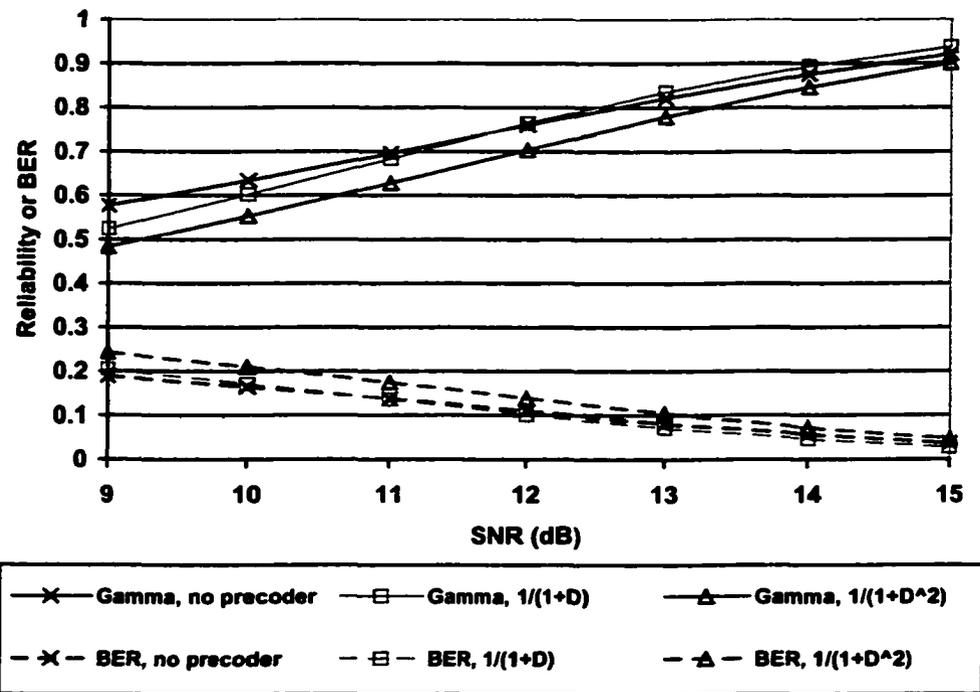
Figure B.2. Mean reliability and BER of equalized EPR4 Lorentzian-Gaussian channel with different precoders,  $S_c = 3.0127$ , AWGN.
