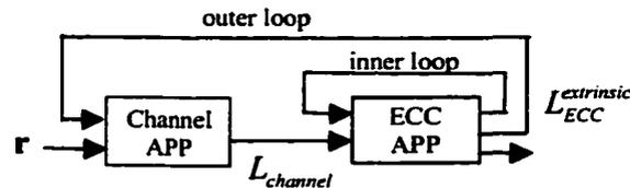
Figure 2.3. Outer and inner loops in an iterative decoding system.
