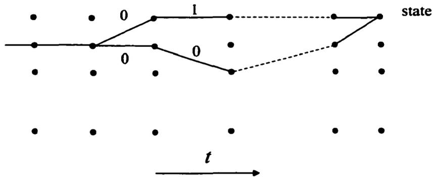
Figure A.1. Trellis diagram for a PR channel.
