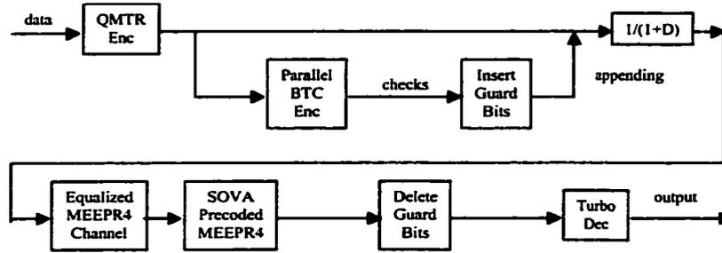
Figure 3.7. Diagram of an equalized ME<sup>2</sup>PR4 MR system with a parallel BTC.
