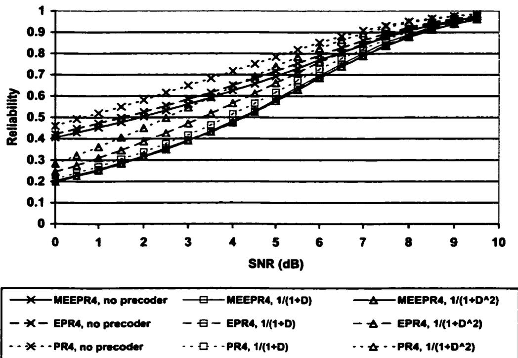
Figure B.1. Mean reliability of ideal PR channels with different precoders.
