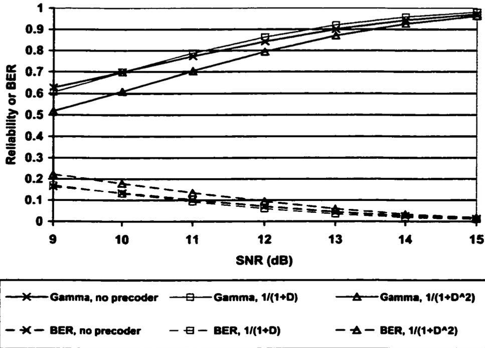
Figure B.3. Mean reliability and BER of equalized ME<sup>2</sup>PR4 Lorentzian-Gaussian channel with different precoders,  $S_c = 3.0127$ , AWGN.
