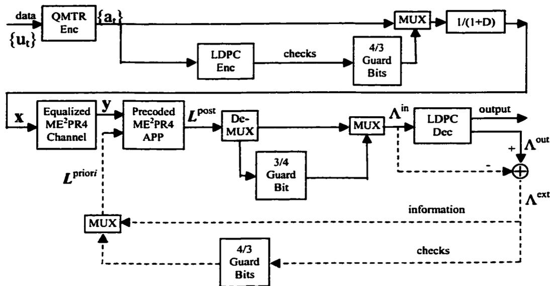
Figure 4.5. Block diagram of a PR channel with an LDPC code.
