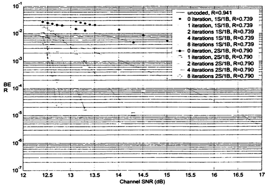
Figure 3.6. BER of equalized EPR4 with a BTC at user density of 2.22.
