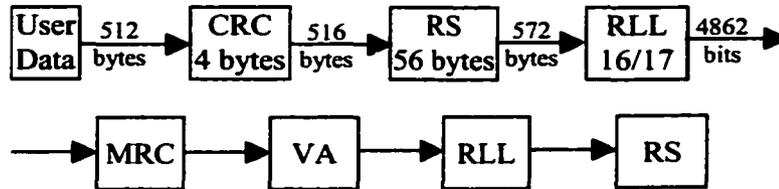
Figure 4.19. System diagram using an RS code.
