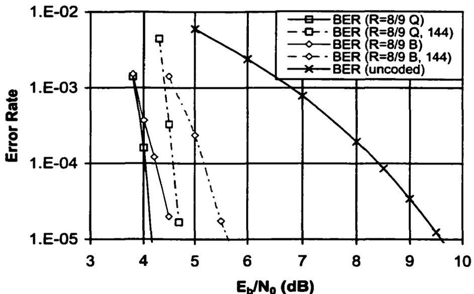
Figure 5.3. Performance of Code 2 and Code B on ISI-free AWGN channels.
