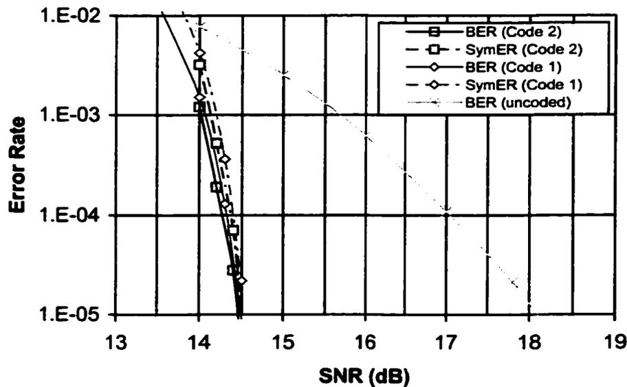
Figure 5.5. Performance of Q-LDPC coded EPR4-equalized MR channel.
