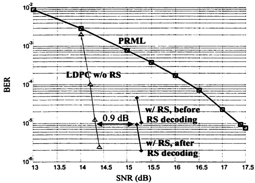
Figure 4.14. Performance of RS-LDPC system taking into account the RS coding penalty.
