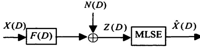
Figure 1.8. All discrete-time channel model.
