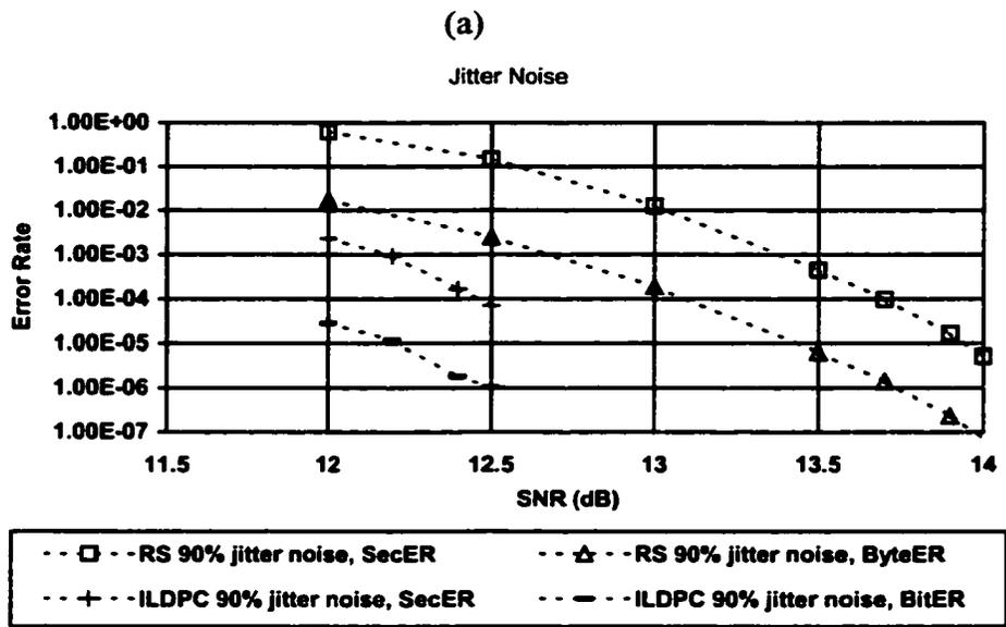
Figure 4.20. Performance of irregular LDPC coded systems. (a) 0% jitter noise;
