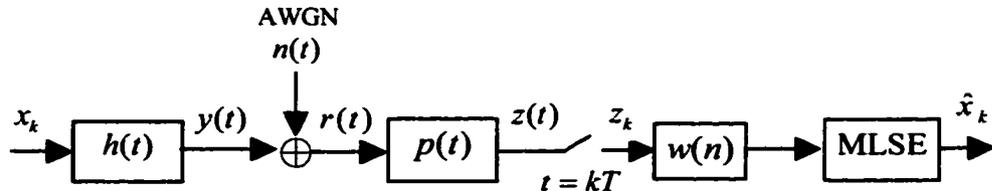
Figure 1.7. Sub-optimal detection with PR equalization.
