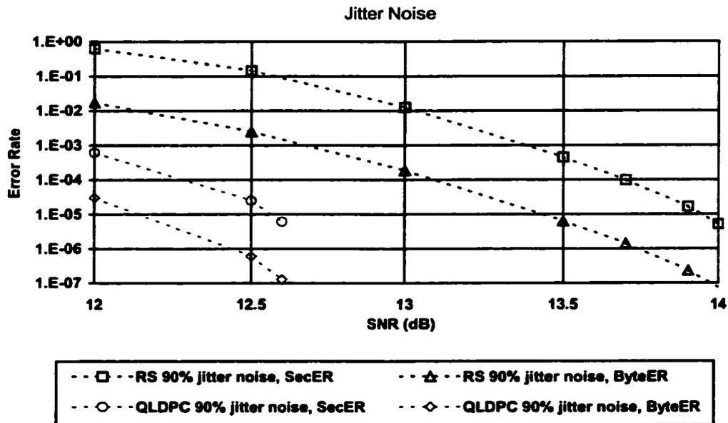
Figure 5.11. Performance on channels with 90% jitter noise power.
