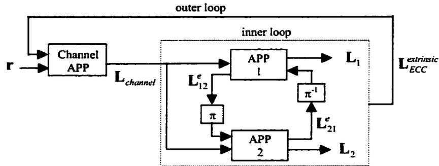
Figure 2.6. Iterative decoding of turbo coded PR channels.
