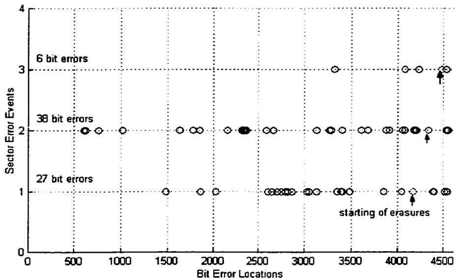
Figure 5.6. Bit error locations of the sectors in error.
