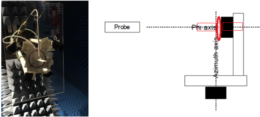
Figure 28: Fabricated E&M Collocated Dipole Antenna and its configuration in NF Chamber (E dipole is aligned along Z axis and Loop is aligned to point Null at the source probe)
