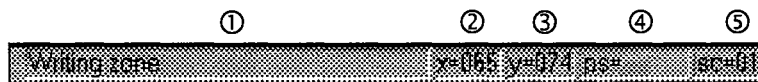
Figure B.7: Status bar and its components. ①: message pane; ②: x coordinate of the pointing device; ③: y coordinate of the pointing device; ④: direction sequence; ⑤: stroke count.
