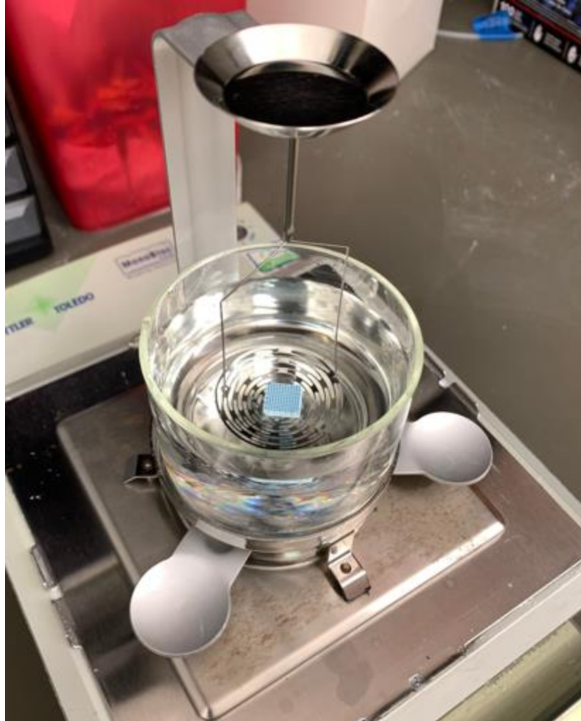
Figure 18: Mettler Toledo Density Kit for Archimedes analysis. Note the submerged scaffold for obtaining m_{\text{submerged}} .
