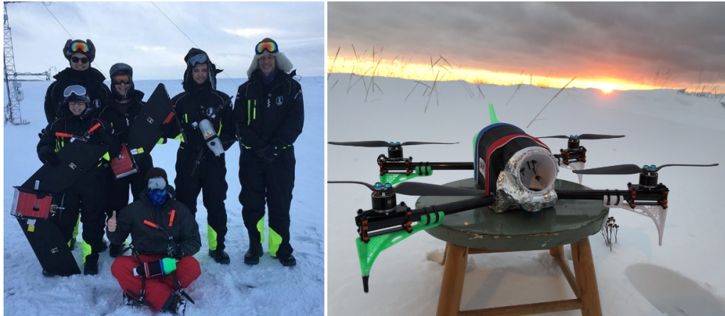
Figure 5.3: Left image: OU-CASS team in the island of Hailuoto, Finland, showcasing the UAS equipment used for the ISOBAR field campaign in February 2018. Right image: Front view of the CopterSonde 2 deployed outside in the freezing environment. This platform was the immediate successor of the CopterSonde-1 and the first design attempt toward the CopterSonde-3D concept. The custom integration of the WVFM and weather sensors into the autopilot were first introduced in this version.
