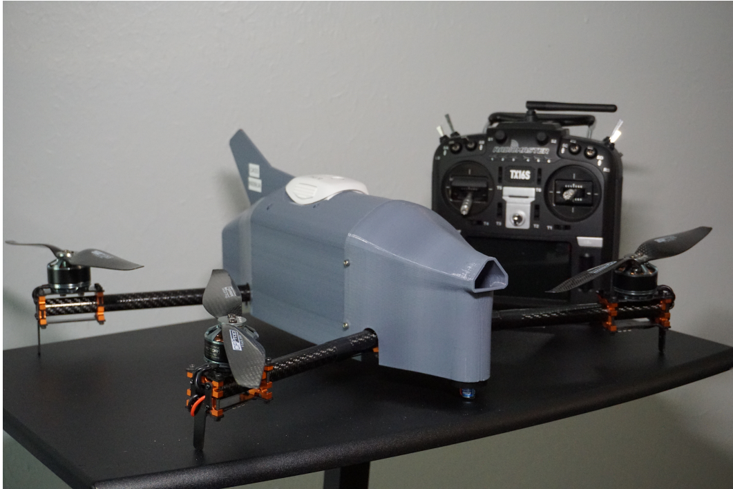
Figure 3.4: CopterSonde-3D concept made in early 2022. A quadcopter UAV specifically designed to collect high-quality thermodynamic observations of the atmosphere. Its peculiar shape is due to the unique arrangement of internal components to improve airflow aspiration across the atmospheric sensors thanks to the addition of a wind vane function to the flight control system.
