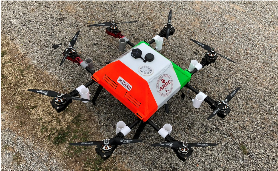
Figure 3.2: CopterSonde-1 concept made in early 2017. An octocopter UAV with temperature and humidity sensors distributed in a symmetrical arrangement around the UAV. The sensors were housed and protected inside plastic tubes and mounted on the UAV's arms below the rotors.
