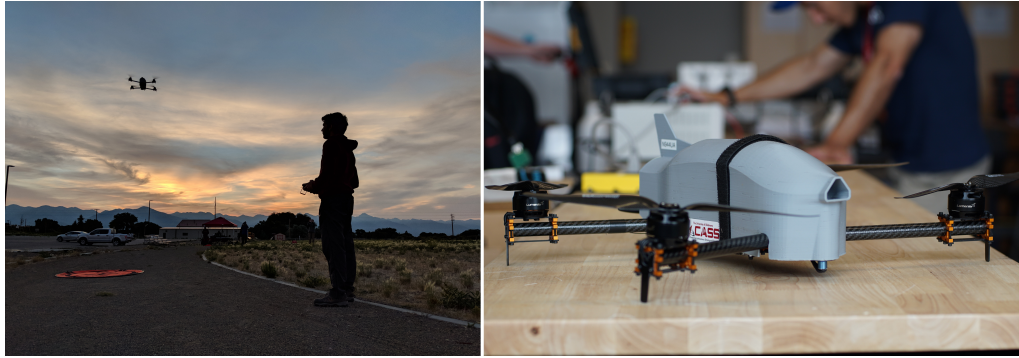
Figure 5.4: Left image: OU-CASS member flying the CopterSonde-2.5 in the San Luis Valley, Colorado, and capturing atmospheric observations for the LAPSE-RATE field campaign in July 2018. The platform successfully flew in an altitude range of 2300–3210 m AMSL for 5 consecutive days. Right image: Front-side view of the CopterSonde-2.5 developed after ISOBAR and first deployed during LAPSE-RATE. The CopterSonde shell was substantially redesigned and streamlined in this version while adding modularity to the payload and other components.
