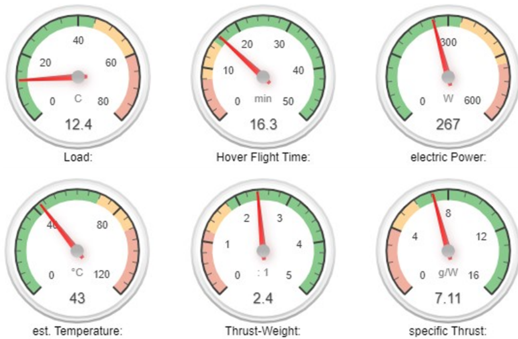
Figure 3.12: Flight performance and efficiency predictions of the CopterSonde-3D using the online Ecalc calculator tool. Each gauge indicates the predicted operating range for the given parameter, where the colors represent levels of risk. Green is ideal, yellow is acceptable, and red is inadequate and may produce unwanted results. Image was taken from Ecalc [94].
