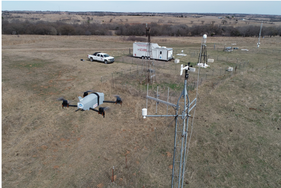
Figure 4.11: Picture of the CopterSonde by the Washington Oklahoma Mesonet tower at KAEFS, near Purcell, Oklahoma. The CopterSonde was flown at a hover at 10 m near the tower for 10–15 min at a time on several days under various wind conditions for the statistical model of wind estimation.
