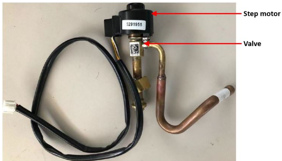
Figure 6.3: CAM EXV (OEM valve used in the test heat pump).
