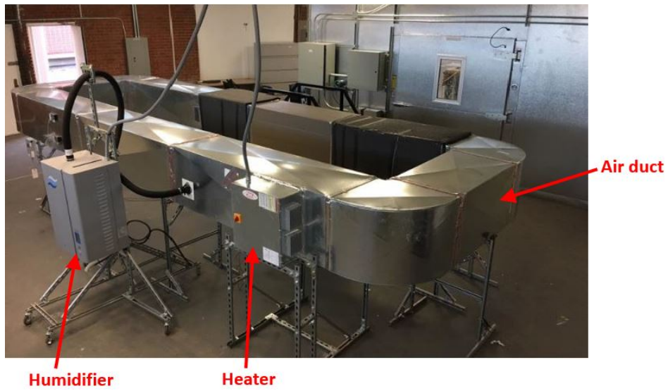
Figure 3.2: Indoor environment test loop.
