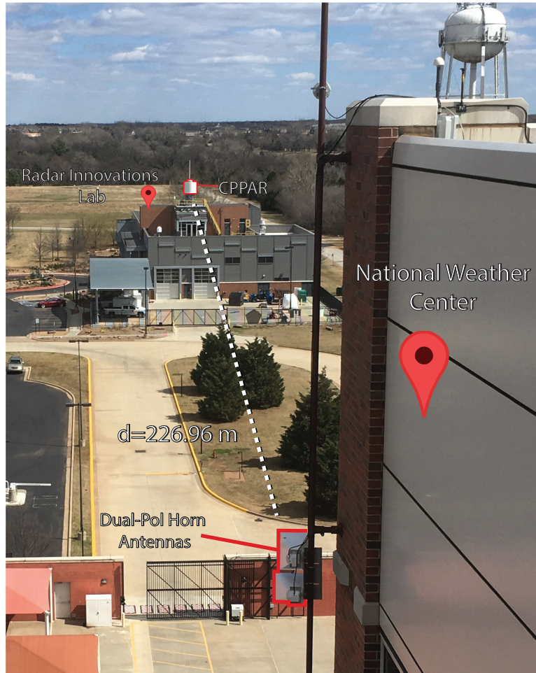
Figure 3.2: CPPAR and the far-field measurement probe (horn shown in the foreground of the picture) [26]. Reprinted from Herndon and Yearly (2021) © 2021 IEEE
