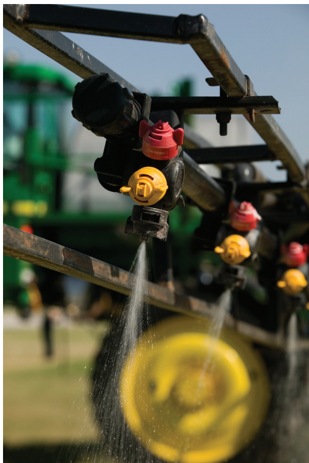
Figure 2. Spray nozzle assemblies consist of a body, cap, check valve, and nozzle tip.
