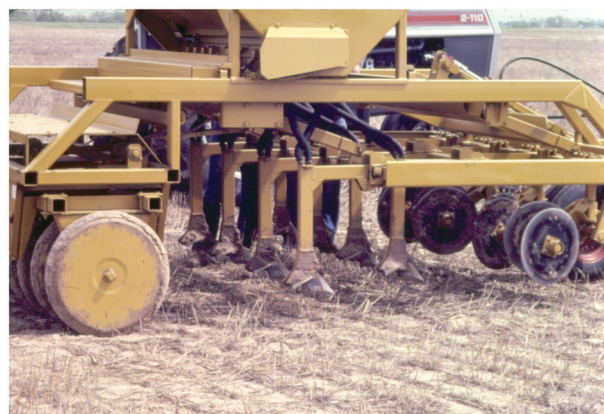
Figure 12. A Haybuster no-till hoe drill. Note the under frame clearance for residue flow.
