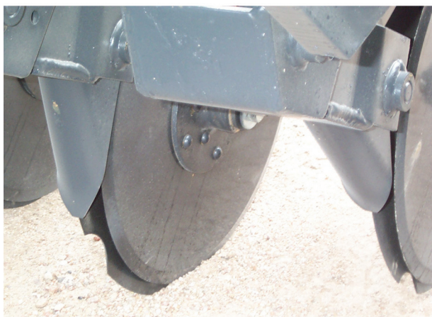
Figure 9. A double disk opener on a no-till drill with staggered disks and a notched leading blade.
