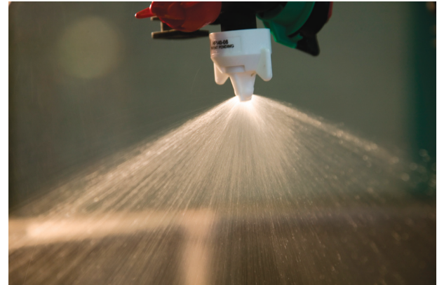
Figure 3. Different nozzles create droplet patterns used for a variety of purposes. (Refer to Table 1 for droplet size categories.)
