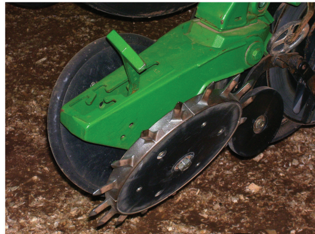
Figure 21. A spike closing wheel used with a standard John Deere closing wheel.
