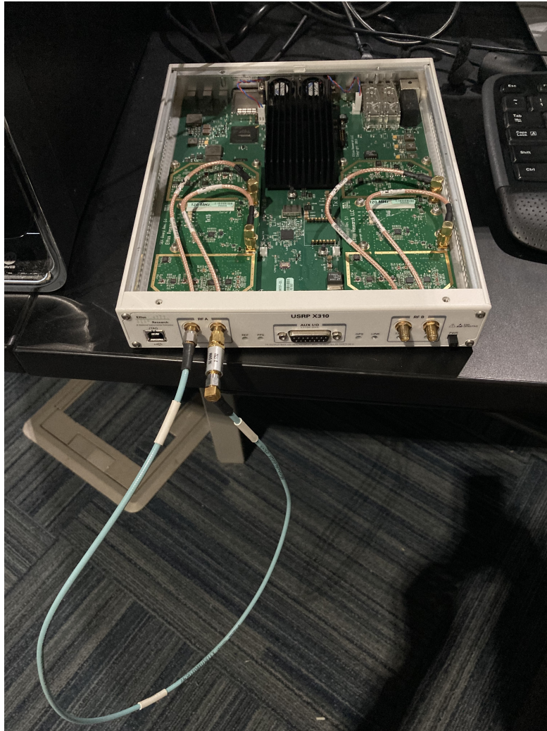
Figure 5.1: Physical setup of the software defined radio testbench.
