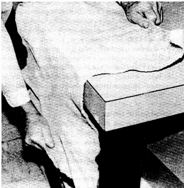
Figure 6. Work the hide over a wooden edge until the stretching makes it completely soft.
