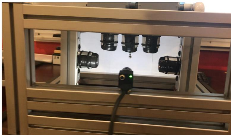
*Figure 20: View of system showing background added for the camera*
