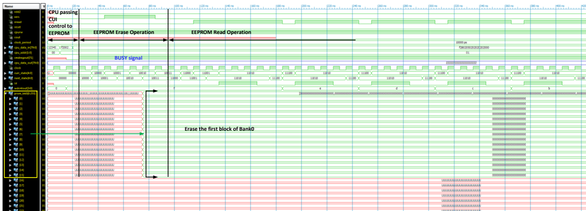
Figure 7.4 EEPROM erase operation. Control transition from CPU to EEPROM. Operation transition from erase to read.
