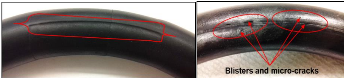
Figure 5.1: Surface defects on elastomer seal resulted in failed leakage tests (Ahmed et al. 2019)
