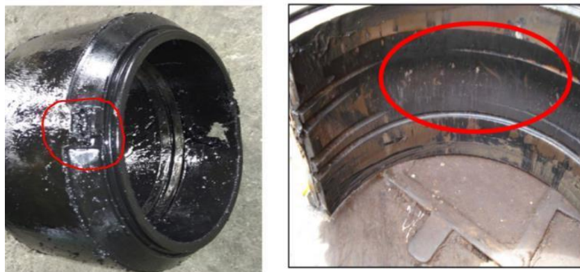
Figure 2.22: Failure in backup ring causing extrusion of elastomer element in packer equipment (Humphreys and Ross 2009)
