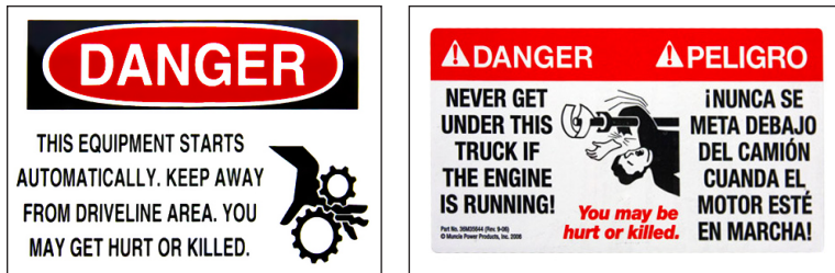
Figure 3. Two examples of warning signs that warn about the dangers of moving parts.
