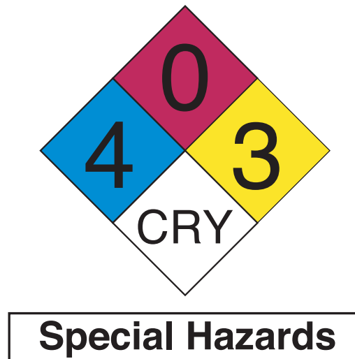
Figure 6. This sign uses color to represent different kinds of hazards to emergency personnel that have learned their meaning.
