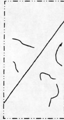
Figure 3-13 Typical Failure of Lime-Stabilized Soil Sample (After ASTM, 1998b)
