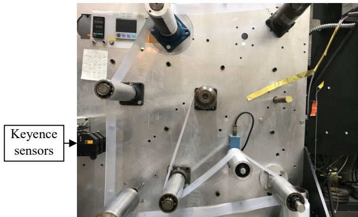
Figure 11 – On-line measurement of CMD Curl
